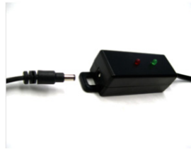
Un-lighted Jumper plugs into Red/Green Lead box
